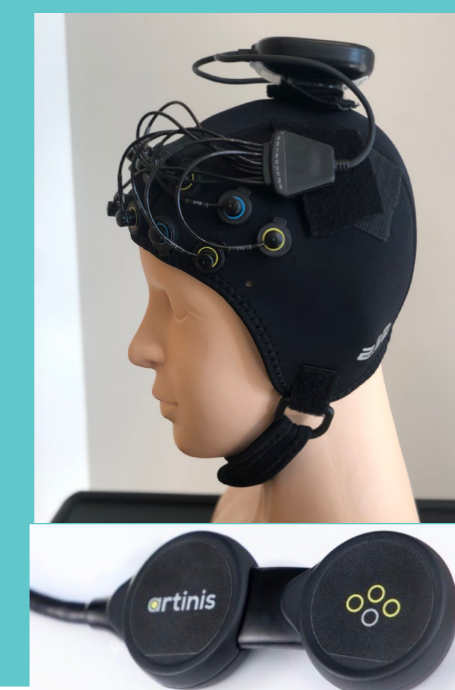
Figure 2. Brite fNIRS brain headcap with emitters and receivers over prefrontal cortex. Portalite NIRS device for positioning over anterior bladder wall.
